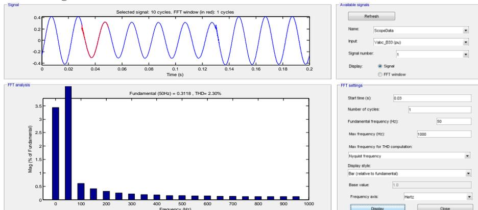
Fig. 9. FFT output of total harmonic voltage distortion
