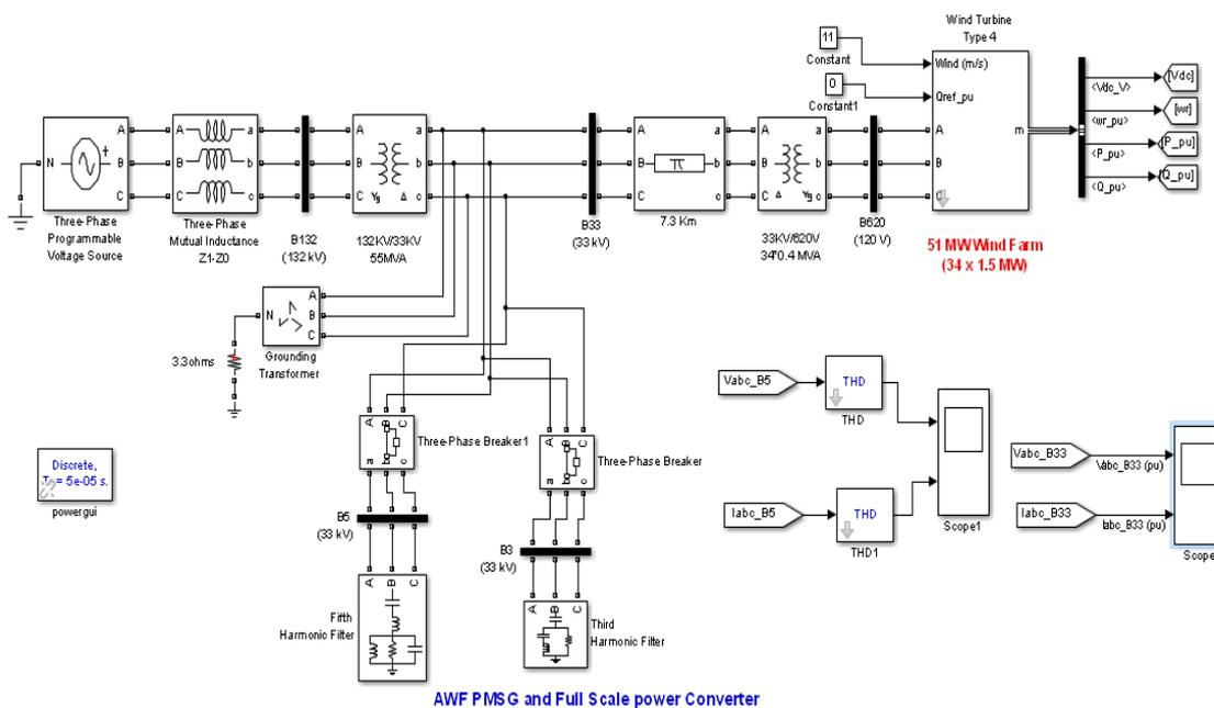
**Fig.6.** Simulink Block diagram of AWF
