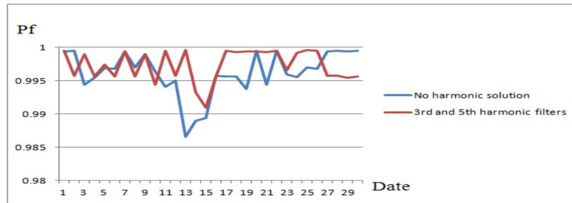
Fig. 12. Harmonic Filters impact on power factor improvement
