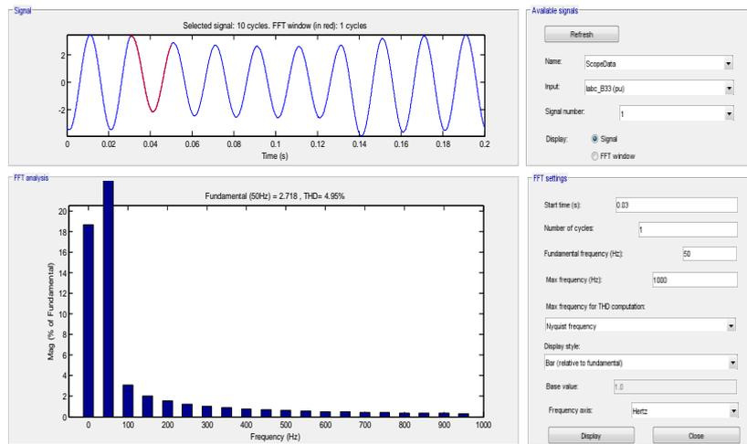
Fig. 8. FFT output of total harmonic current distortion
