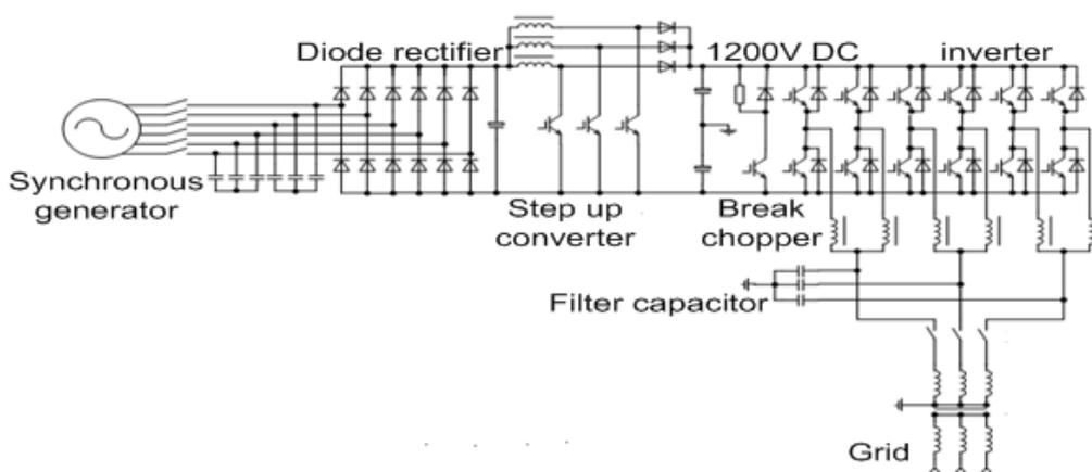
Fig.2. Six phase converter inverter system of AWF [5]
