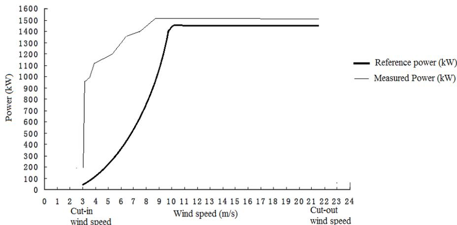
Fig.4. Comparison between the reference and measured power curve.
