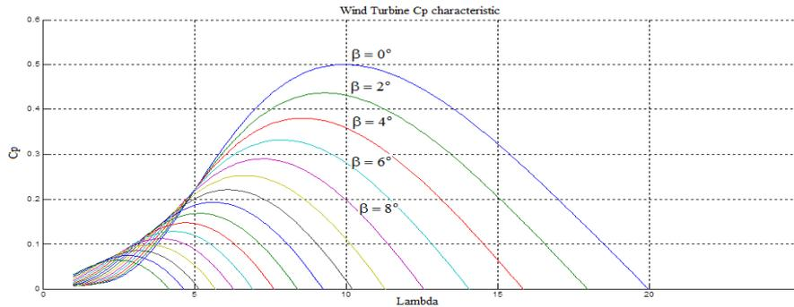
Fig.3. Cp Vs λ output at different pitch angle.
