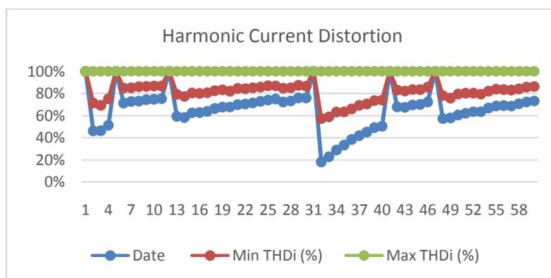
**Fig. 10.**Summary of current THD at 33 KV bus bar system
