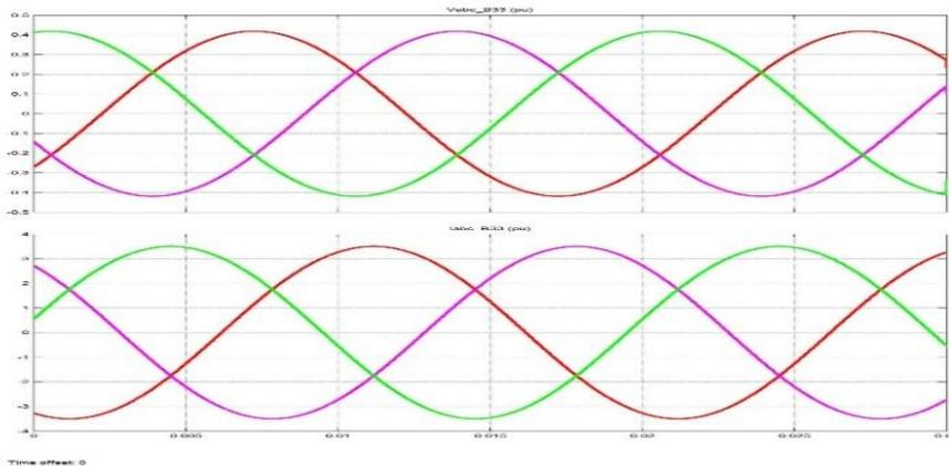
Fig. 7. V and I three phase wave form output at 33 KV busbar
