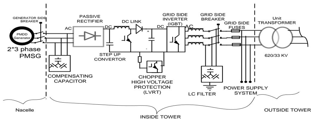
Fig. 1. Gold Wind 1.5 MW Electrical Diagram [5]
