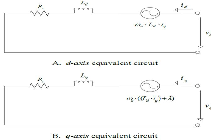
**Fig.5.** Equivalent circuit of PMSG in d-q reference frame
